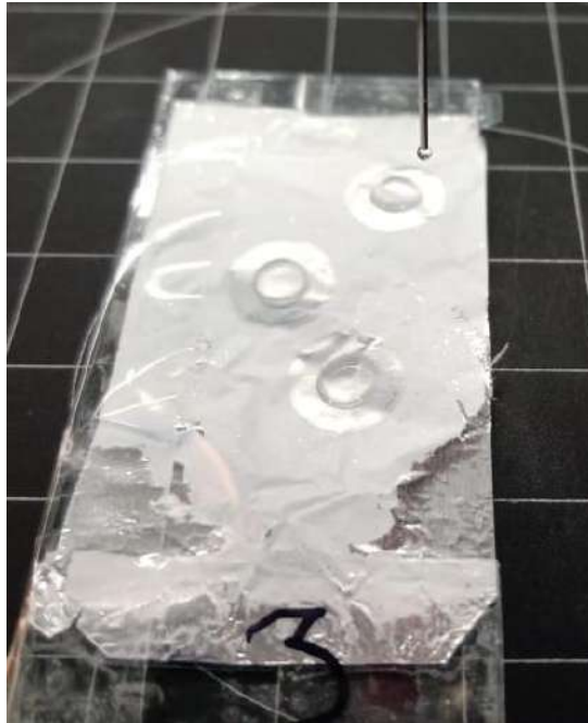
Figure 12: Fibrous mats with water drops during contact angle tests
