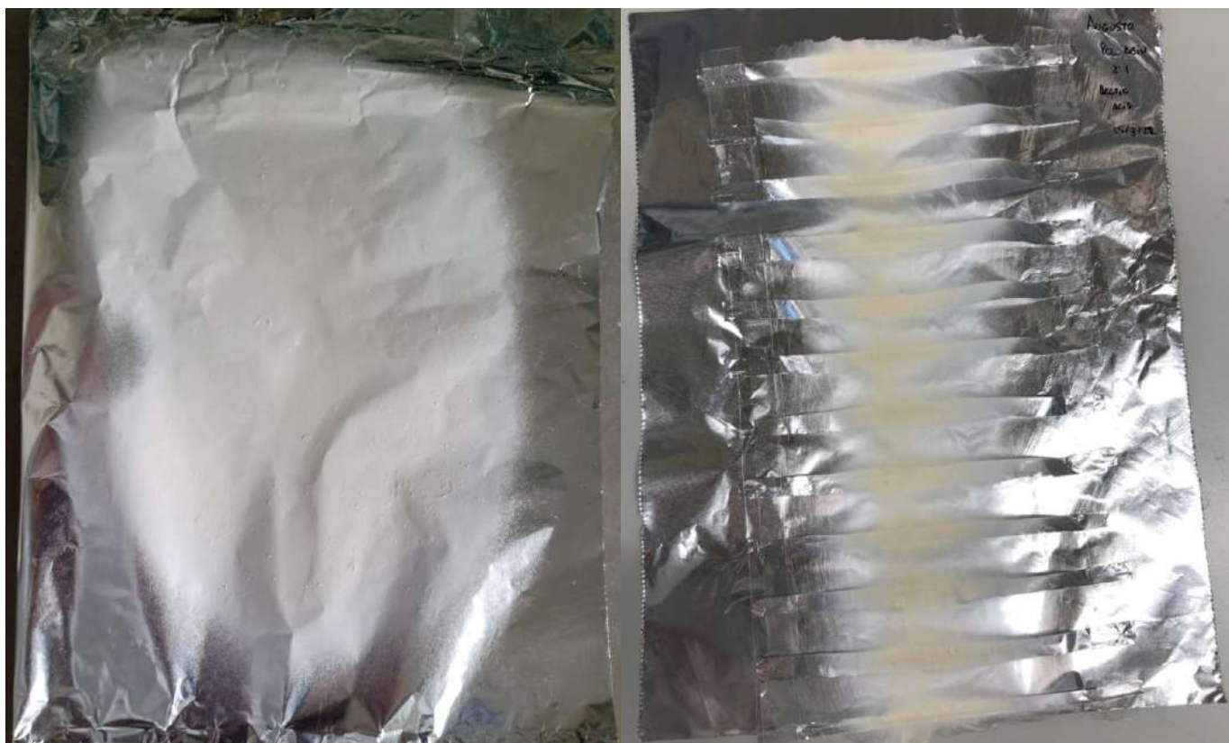
Figure 9: The influence of collectors on the final structure of the fibers. (a) typical random fibrous mat, (b) aligned fibers.
