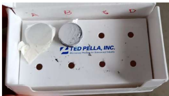
Figure 10: Plates for samples for SEM examination
