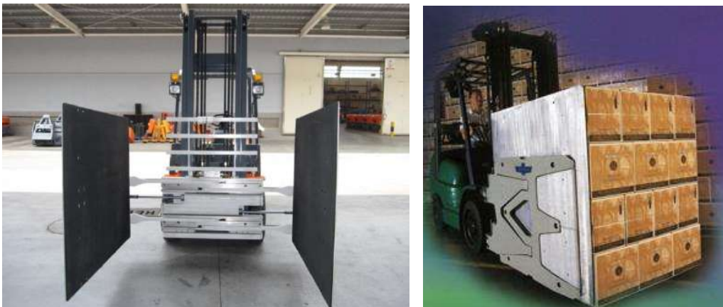
Figura 24- Clamp para cargas a granel de cajas (TOYOTA Industrial Equipment, 2017)
