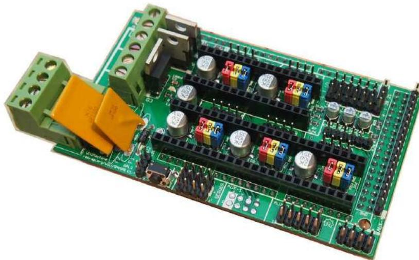
Figura 20: *RepRap Arduino Mega Pololu Shield* (RAMPS 1.4)
