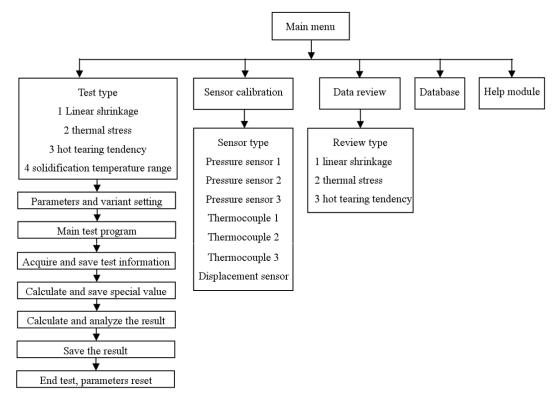
Fig.6: Framework of solidification characteristics test module
