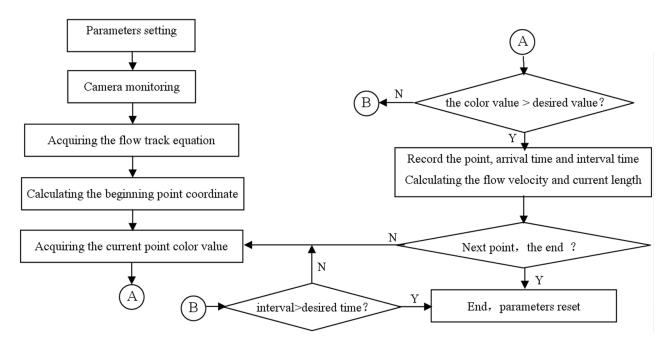
Fig.5: Main program of calculating the flow velocity and length based on flow track
