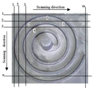
Fig.1: Order of the points based on scanning
