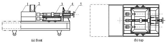
1 modeling units, 2 thermal analysis sampler, 3 sensor group, 4 positioning units, 5 unloading units
