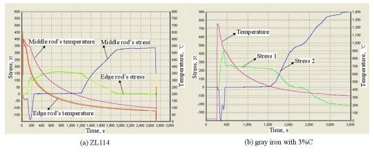
Fig.8: Stress-time relation of different alloys
