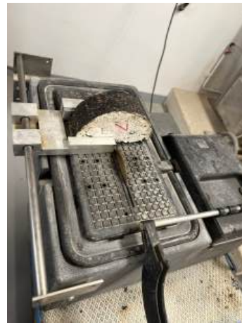
(b) Equipment used for creating the cracks of the specimens.
