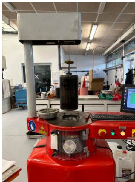
Figure 2.4: PCG machine with mould containing asphalt mixture.
