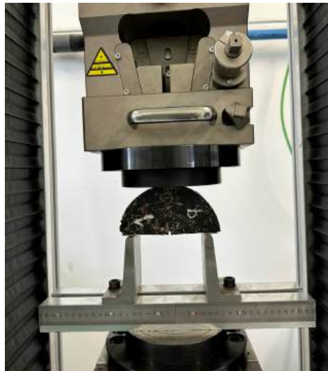
Figure 2.13: Arrangement of SCB specimens.
