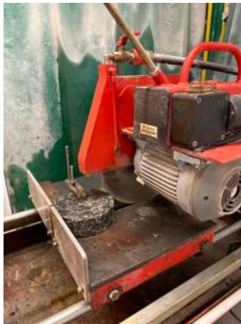
(a) Equipment used for cutting the semi-circle and prismatic specimens.
