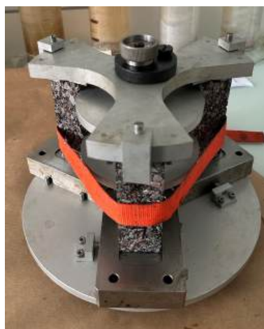
Figure 2.10: Equipment used for gluing the stiffness specimens.
