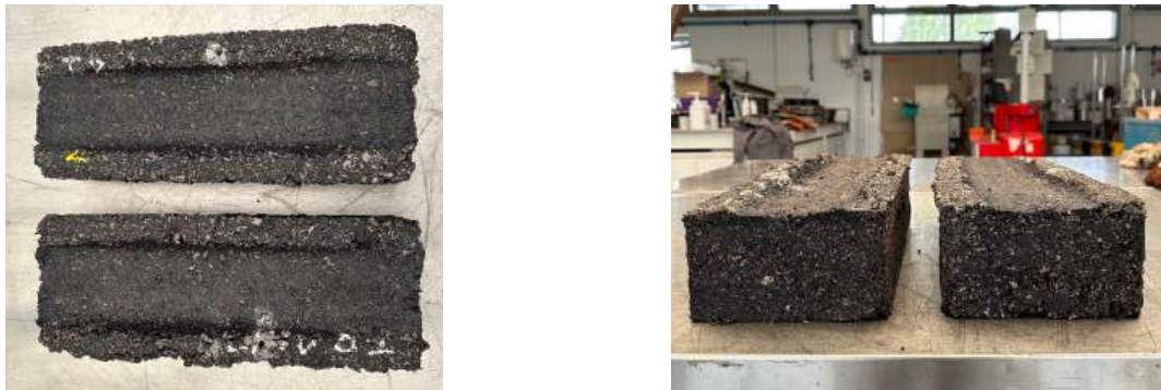
Figure 3.11: Rutting specimens after testing.
