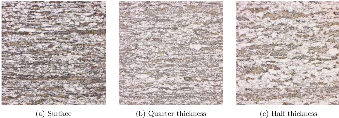
Figure 4.40: Microstructural gradient. Sample 1317, 500x magnification, Zeiss Axio Imager.M2m, optimal imaging settings.
