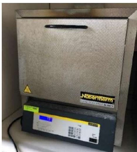
Figure 6 – Nabertherm P330 used for calcination
