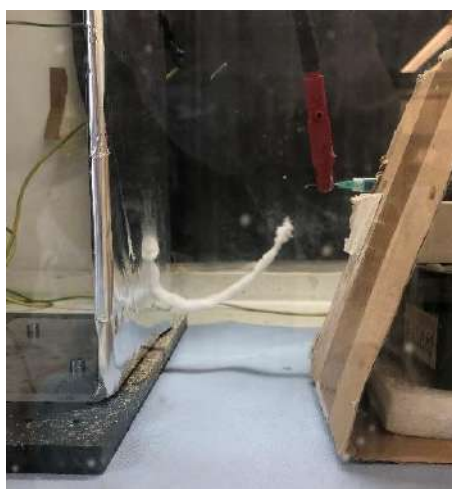
Figure 5 – Nanofibers production using ES
