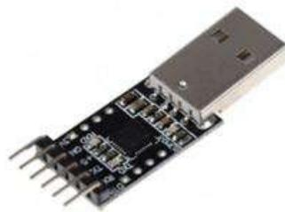
FIGURA 3.44: Conversor USB - UART TTL.
