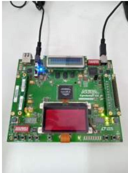
Figura 3.3: FPGA Cyclone III - Altera
