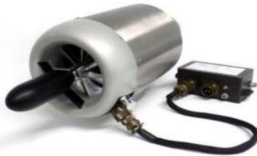
The Lynx is a "spin-off" of the AMT-NL Nike design and has been constructed from a single radial compressor and a axial flow turbine stage. The engine owns its excellent performance and superb power to weight ratio to our unique 3D diffuser.
