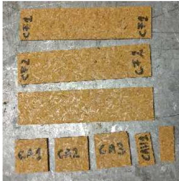
**Figura 2.6.** *Probetas de CA-BSPC.*
