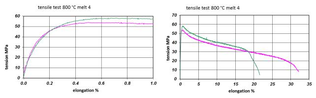
Fig.17 (left) and 18 (right): Result of two tensile tests of melt No. 4 with 5.5 % Si and 2.9 % Al at 800 °C. The tensile strength Rm is 54and 58 MPa (measured at GF central lab with a speed of 0.2 mm/min., according to ISO 6892-2:2011). No values of melt No. 3 available.
