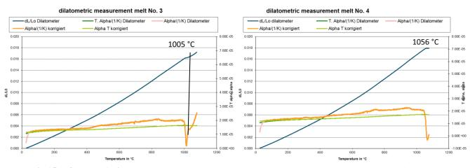
Fig.15 (left) and 16 (right): Dilatometry measurement graphs, indicating the ferrite/austenite transformation temperature of melt No. 3 with 5.3 % Si and 1.96 % Al, and melt No. 4 with 5.5 % Si and 2.91 % Al.
