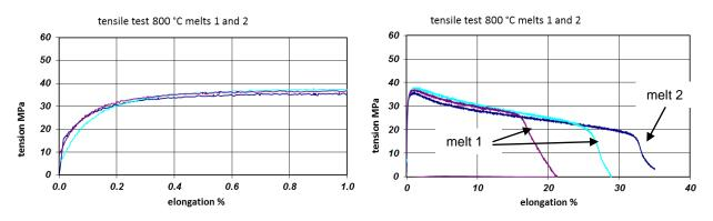
Fig.13 (left) and 14 (right):Result of tensile tests at 800 °C. The tensile strength Rm of melt No. 1 with 1.8 % Co and melt No. 2 with 4.0 % Co is 36 MPa and 38 MPa, respectively.
