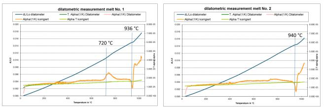
**Fig.11 (left) and 12 (right):** Dilatometry measurement graphs, indicating the ferrite/austenite-transformation temperature of melt No. 1 with 1.8 % Co, and melt No. 2 with 4.0 % Co. The first peak of melt No. 1 at 720 °C is probably due to solution of remaining pearlite.
