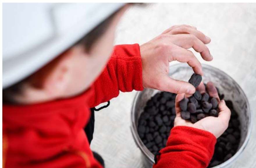
Figure 6. Industrial iron ore pellets. Illustration from AMBARtec. (AMBARtec, 2024)
