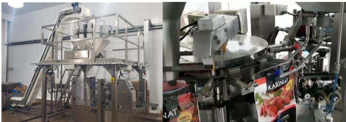
Figura 27: Máquina envasadora DoyPack.
