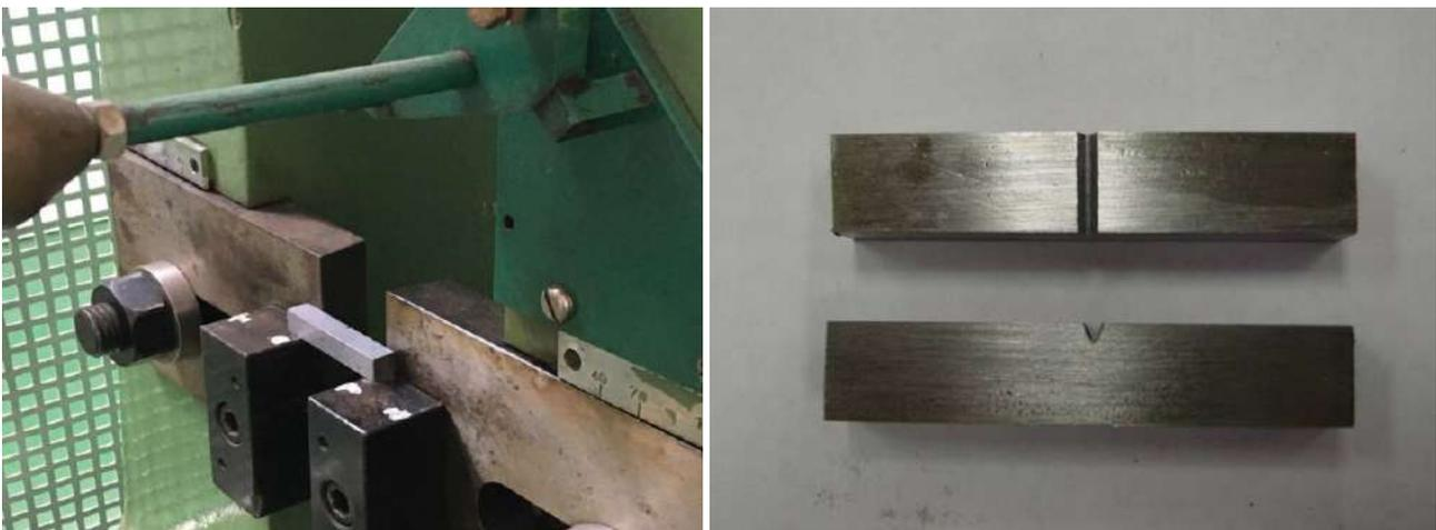
**Figura 11: Probetas Charpy**
