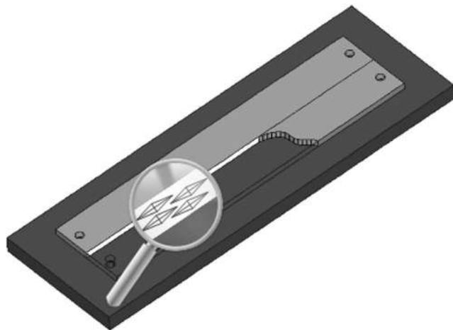
Fig. 3 Location of Knoop microindentations on samples and samples arrangement
