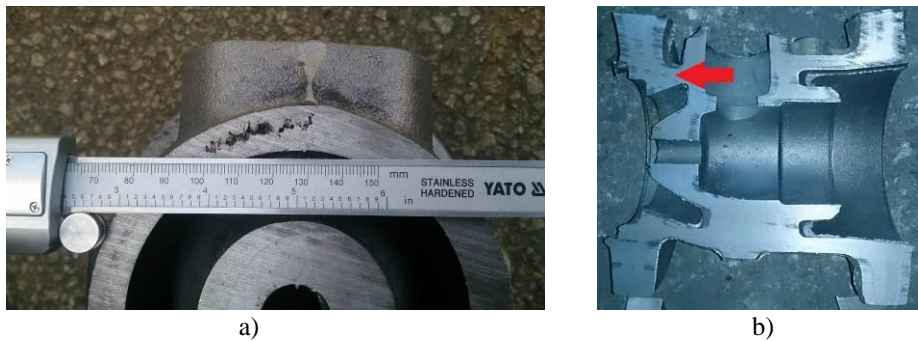
Fig. 1: An example of shrinkage defect in a DI casting (a); a place of the section indicated by the arrow (b).
