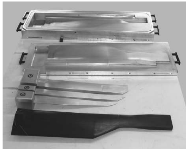
Figure 2.16. Manufacturing moulds for a helicopter tail rotor made from CFRP [71]
