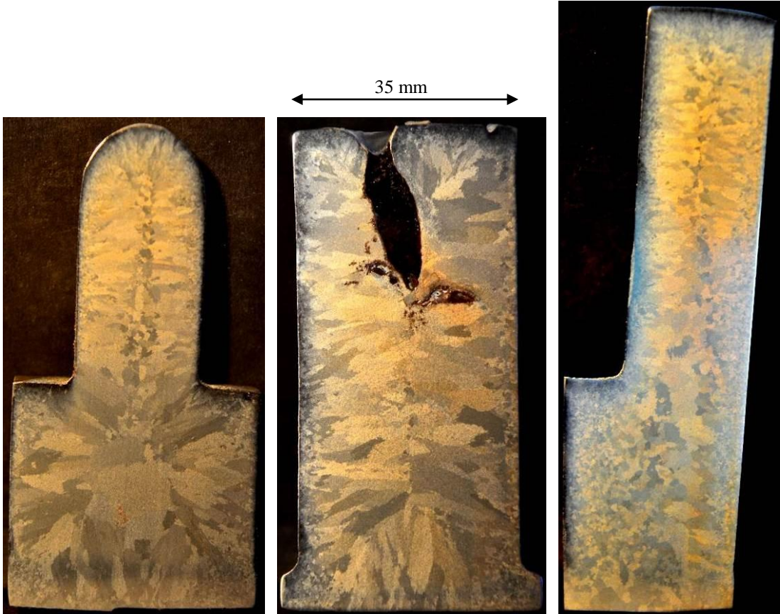
Fig. 7: Solidification macrostructures obtained for Melt A.
