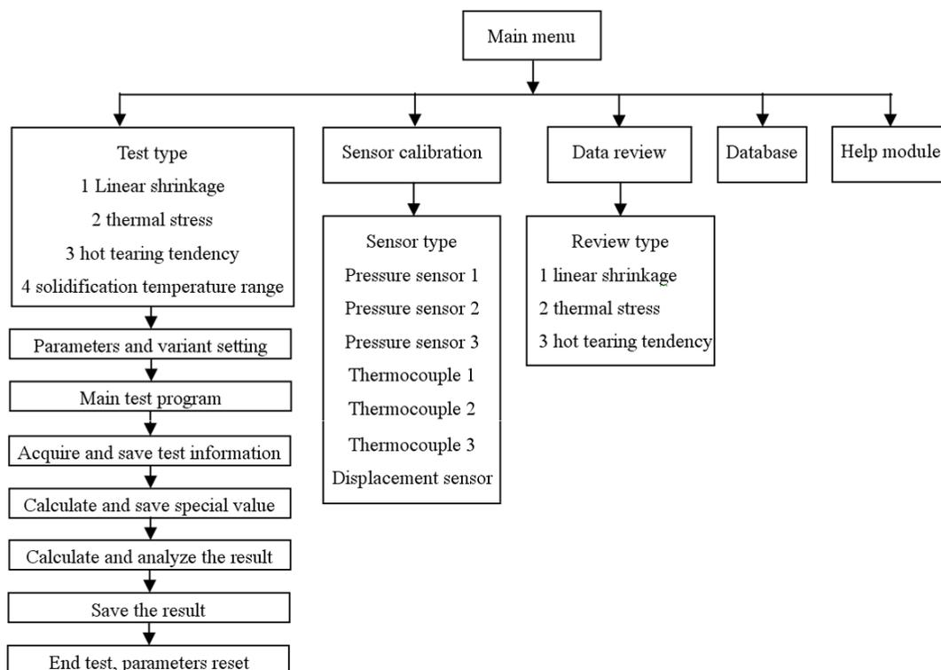
**Fig.6:** Framework of solidification characteristics test module
