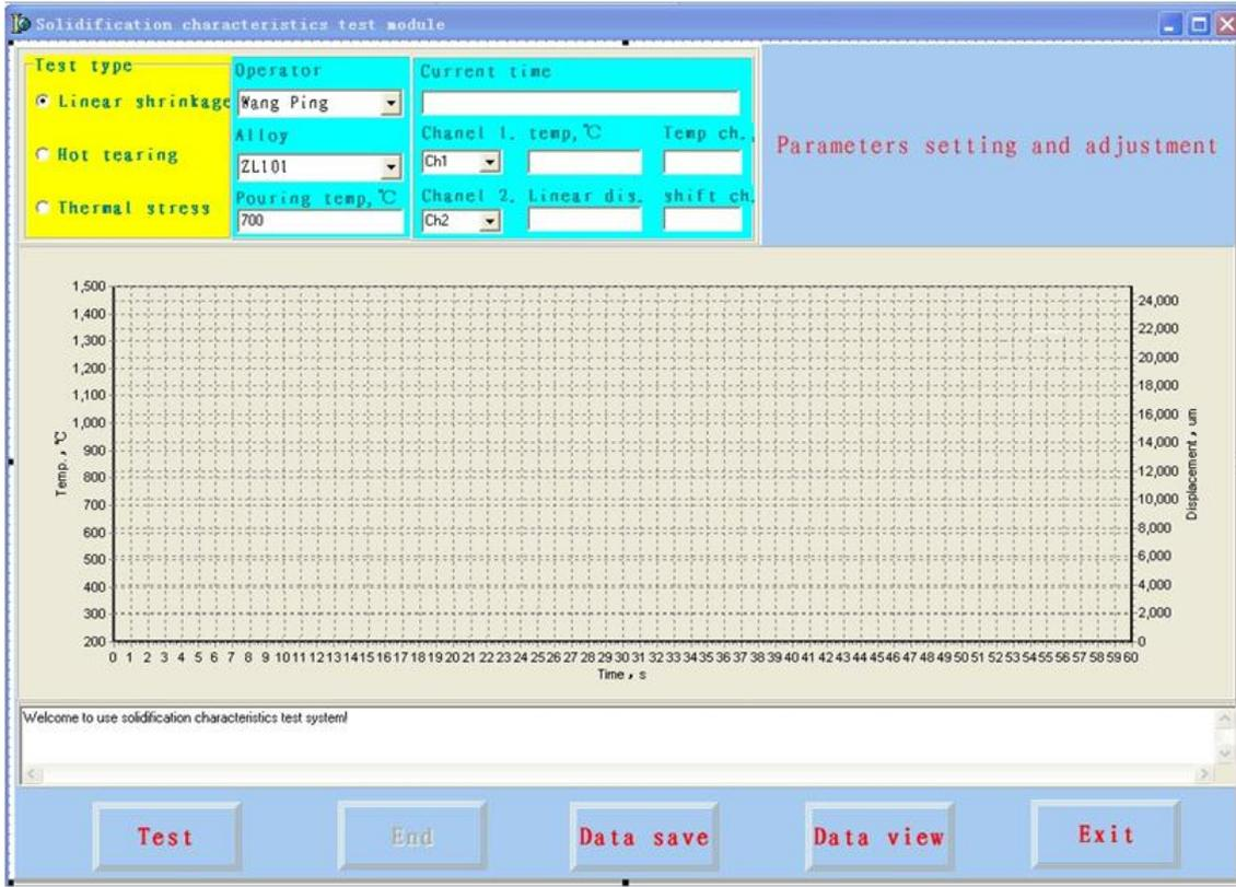
Fig.7: Main program interface of solidification characteristics test module
