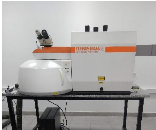
Figura 3.6 - Microscopio Raman (Renishaw RM 2000, UK)
