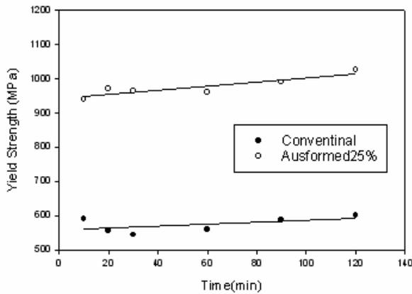
Fig. 5: Yield strength vs austempering time and ausforming reduction for adis alloyed with 2% Ni<sup>47</sup>
