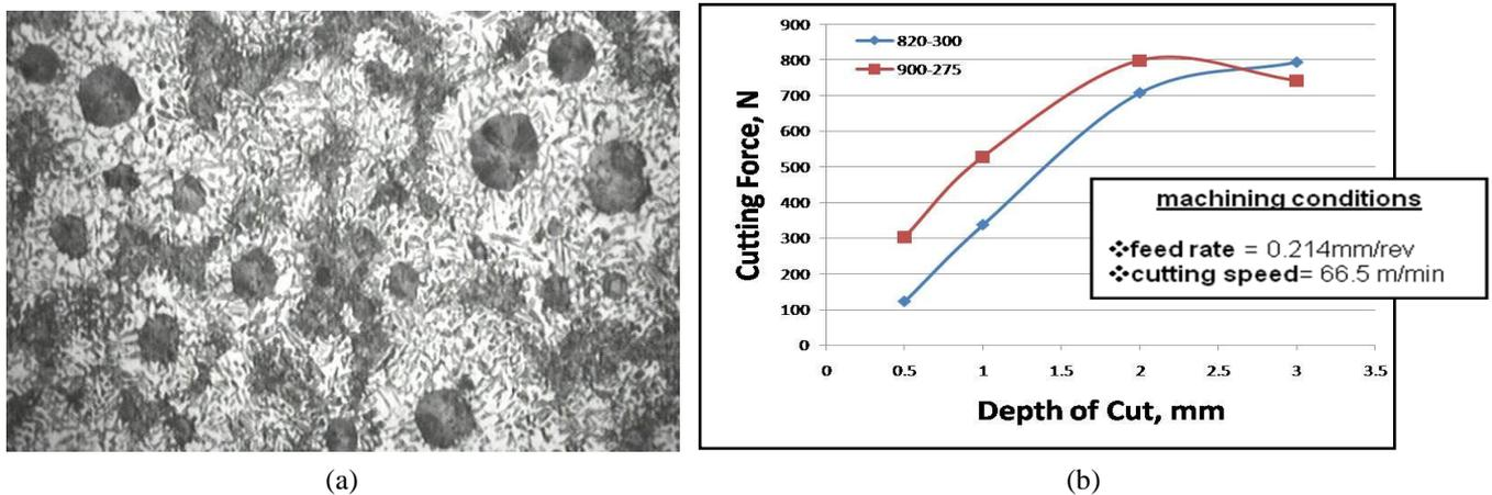
**Fig. 8:** (a) The microstructure of IADI austenitized at 820°C and austempered at 375°C.
