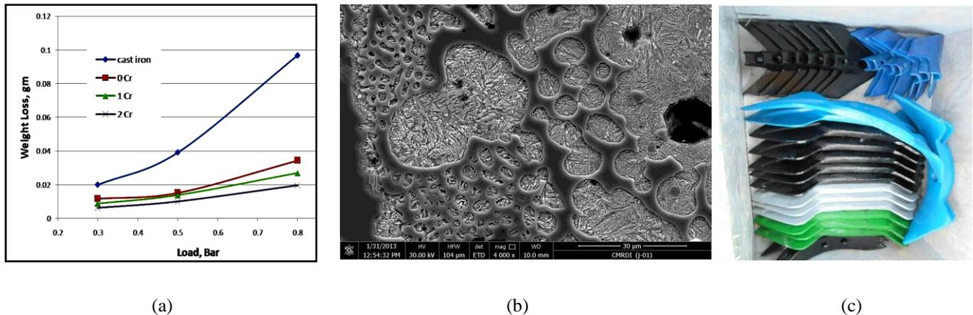
**Fig.1<sup>25</sup>:** (a) effect of Cr% on the wear resistance of CADI
