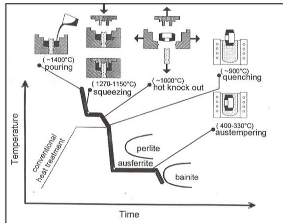
Fig. 6: Process steps and temperature regime of the SQ process and the in-situ heat treatment<sup>52</sup>
