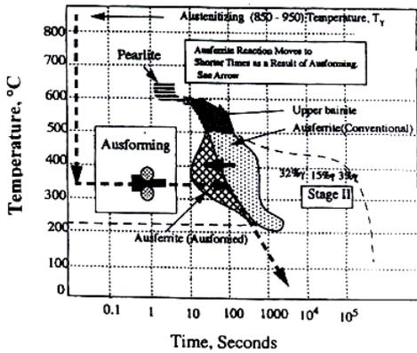
Fig. 3: Schematic representation of the ausforming process<sup>42</sup>
