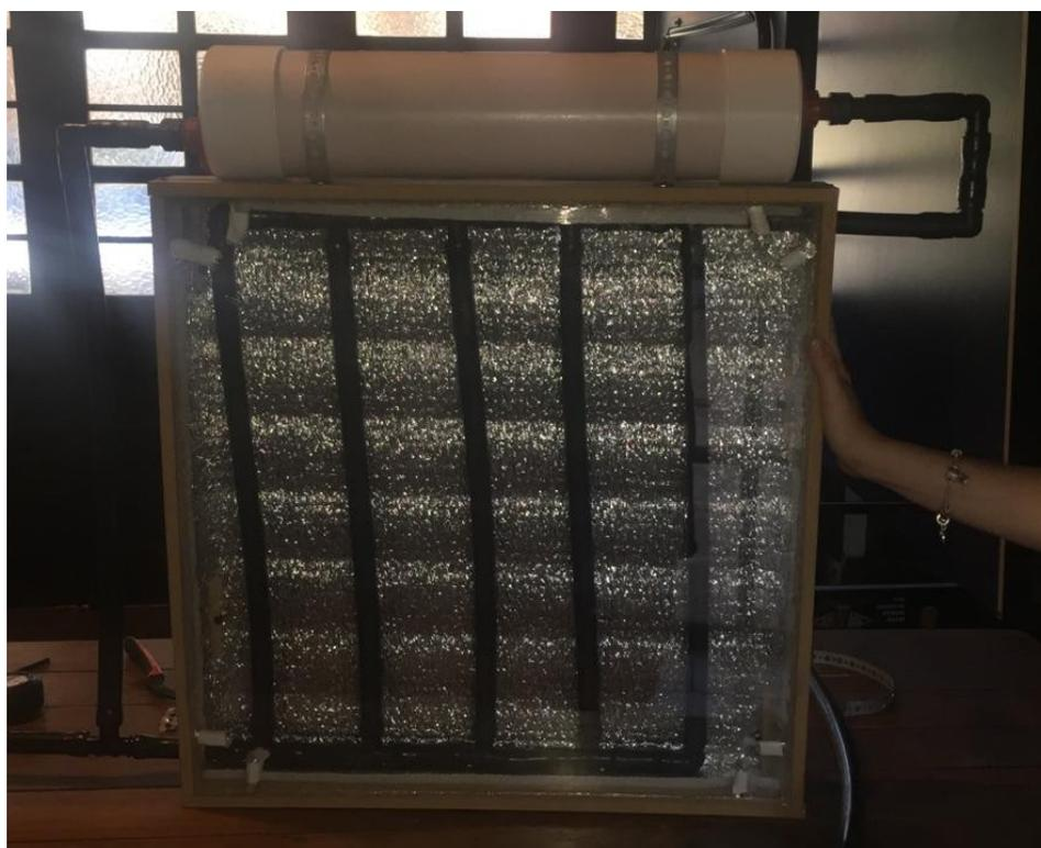
Figura 14. Colector Placa Plana 0.6x0.6 m
