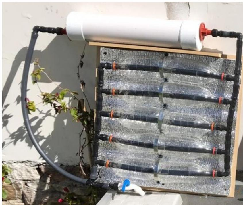
Figura 13. Colector PET 0.6x0.6 m
