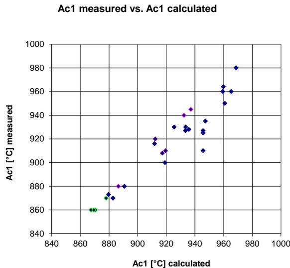
**Fig.3:** Correlation between calculated and measured ferrite/austenite transformation temperatures
