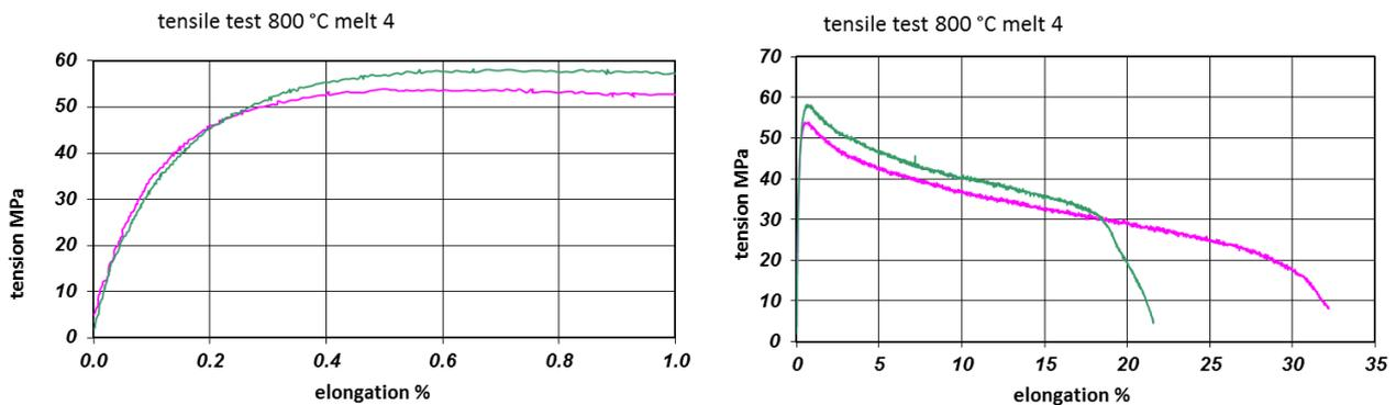
**Fig.17 (left) and 18 (right):** Result of two tensile tests of melt No. 4 with 5.5 % Si and 2.9 % Al at 800 °C. The tensile strength Rm is 54 and 58 MPa (measured at GF central lab with a speed of 0.2 mm/min., according to ISO 6892-2:2011). No values of melt No. 3 available.
