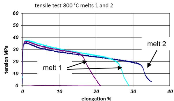
**Fig.13 (left) and 14 (right):** Result of tensile tests at 800 °C. The tensile strength Rm of melt No. 1 with 1.8 % Co and melt No. 2 with 4.0 % Co is 36 MPa and 38 MPa, respectively.
