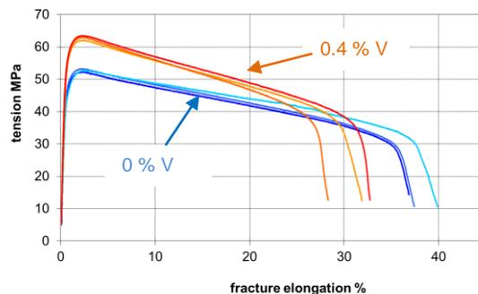
**Fig.9:** Result of tensile tests at 800 °C: significantly higher tensile strength with 0.4 % V (measured at ÖGI with a speed of 0.3 mm/min, according to ISO 6892-2:2011 .)
