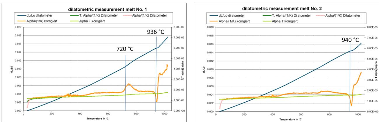
**Fig.11 (left) and 12 (right):** Dilatometry measurement graphs, indicating the ferrite/austenite-transformation temperature of melt No. 1 with 1.8 % Co, and melt No. 2 with 4.0 % Co. The first peak of melt No. 1 at 720 °C is probably due to solution of remaining pearlite.
