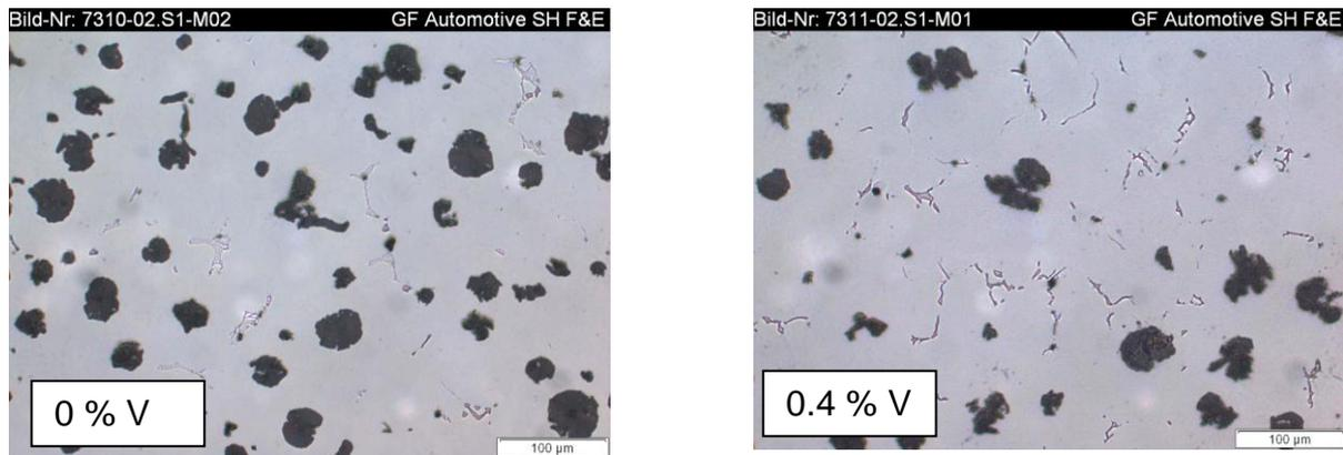
**Fig.7(left) and 8 (right):** Micrographs of the two variants without V (left) and with 0.4% V (right). The experiment confirms the predicted higher amount of carbides with 0.4 % V.
