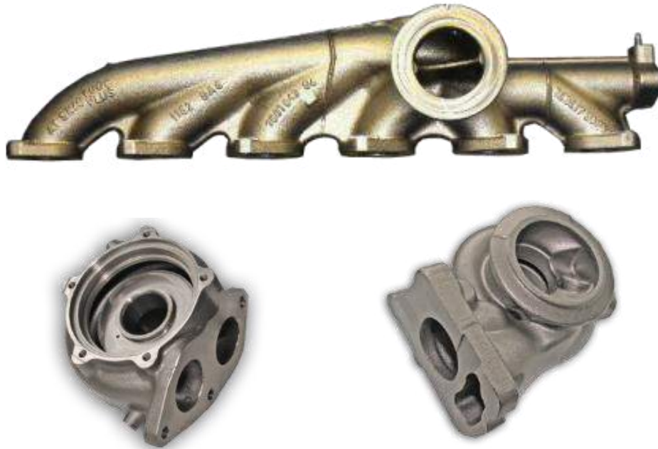
Fig.1: Examples of a serial exhaust manifold and turbocharger housings made of GJS SiMo1000.
