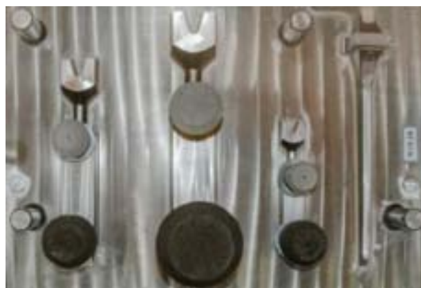
Fig.3: Spot feeders from group 6 mounted on the pattern, ready for moulding. Insulating spot feeders on the top. Exothermic spot feeders at the bottom.
