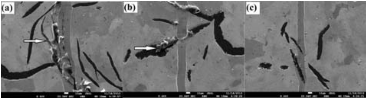
Fig. 6: Interaction between a single scratch pass made by Vickers micro-indenter, and graphite lamellas with different orientations with respect to the indenter tip.
