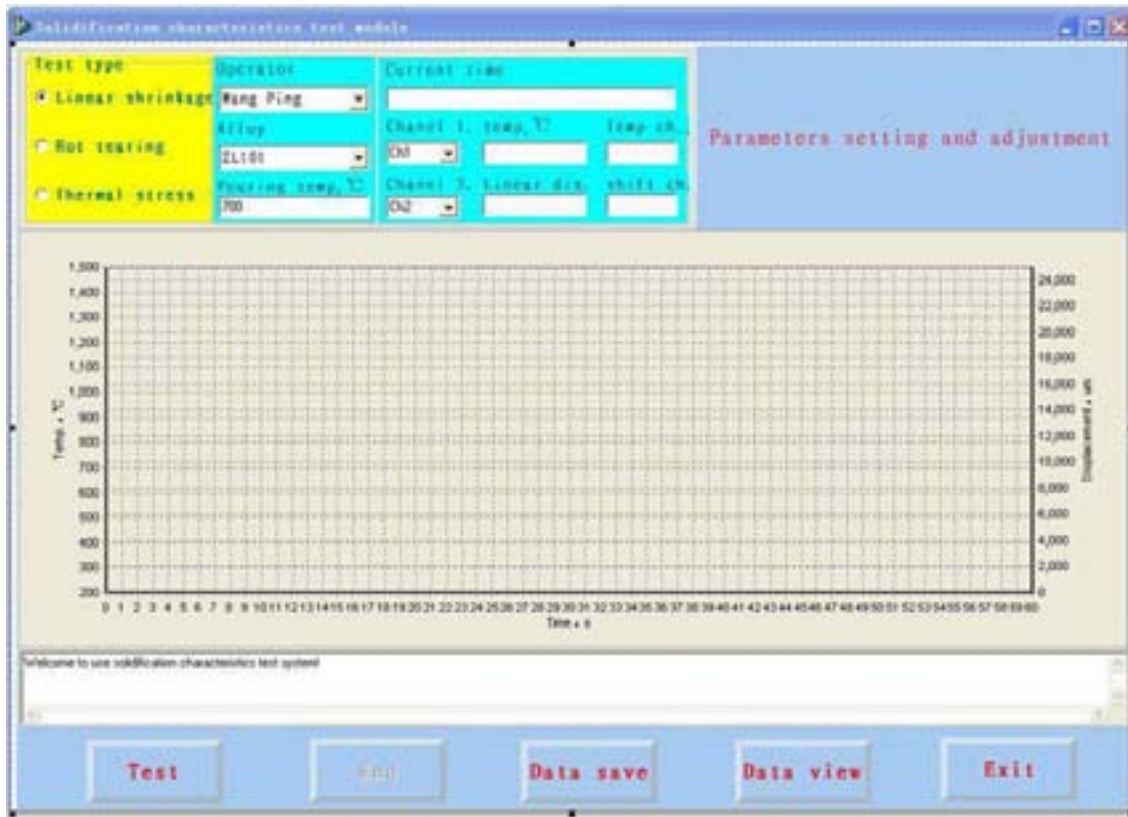
Fig.7: Main program interface of solidification characteristics test module
