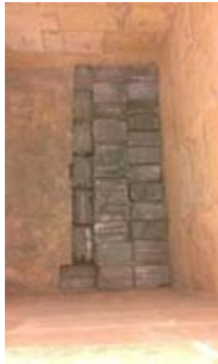
Fig.8: Inoculant in the large pouring basin.
