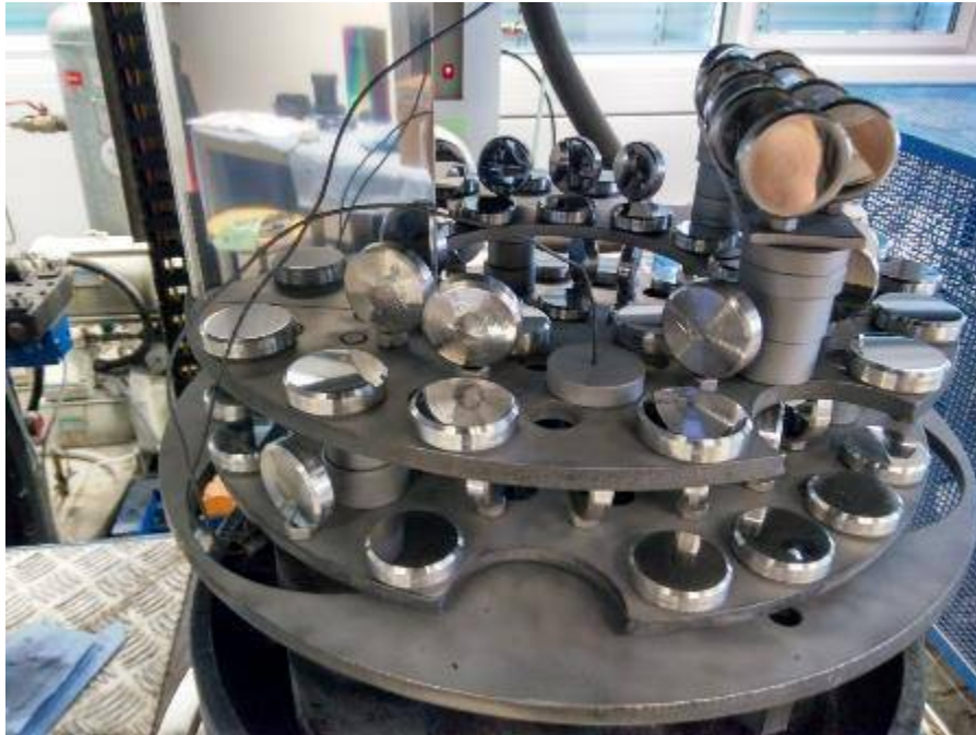
Figure 15. Reactor loaded with polished AISI 304 samples before nitriding process starts.
