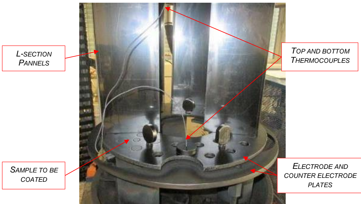
Figure 17. Layout of a typical PACVD process in FHÖO.
