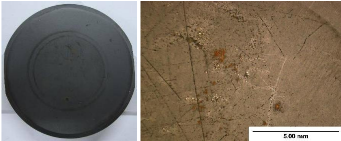
Figure 55. Reddish corrosion products on the AS-TN-NSi-NIL-N sample's surface after the 50-hour immersion test.
