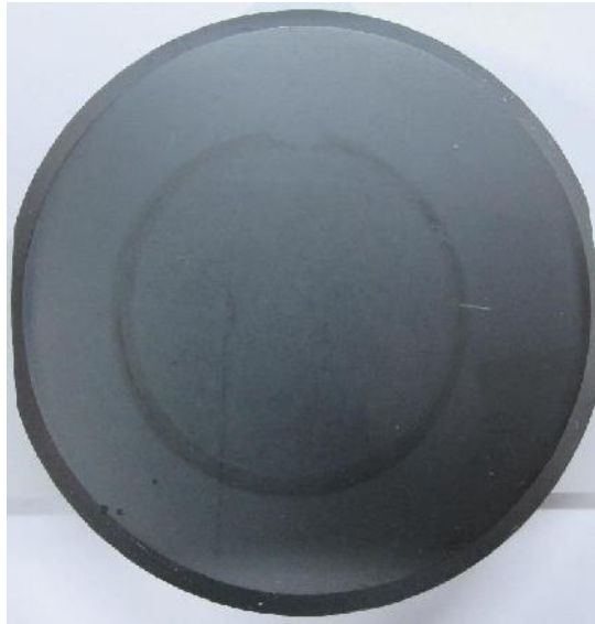
Figure 30. DLC coated sample after immersion test was performed.
