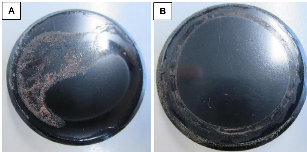
Figure 87. A) SS-N-NiL-TN-Si 300-hour sample after the salt spray test. B) SS-TN-NSi-IL-N 300-hour sample after the salt spray test.
