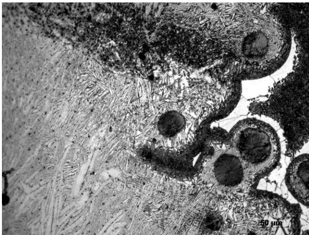
Fig.4: microstructure at the upper part of the HAZ or transition zone
