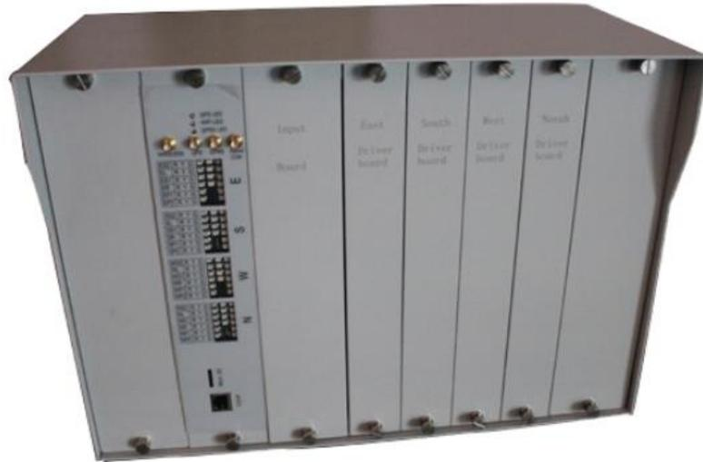
Figura 0.1 – Controlador 2nd generation controller system de Shenzhen Noble Opto Co.
