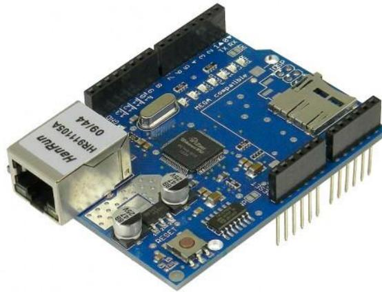
Figura 3.1.3.2.1 – Shield Ethernet W5100
