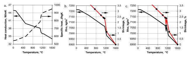
**Fig.3:** Chosen database parameters for EN-GJL-250 cast iron: a. heat conduction and specific heat, b. density and shrinkage curves in variant Rho 1 (without graphite expansion consideration), c. density and shrinkage curves in variant Rho 2 (with graphite expansion consideration).
