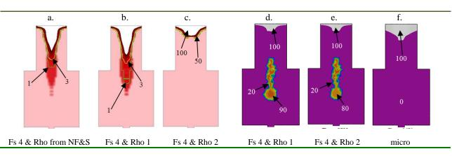
Table 5: Final shrinkage from NF&S CV (a,b,c) and ProCast (d,e,f) for chosen cases – cube casting (shrinkage %).
