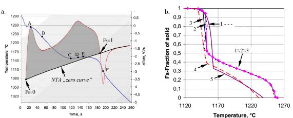
**Fig. 2a:** Cooling curve of grey cast iron type EN-GJL-250 and its first derivative obtained by DerTA cup method (ITACA<sup>14</sup>) with principle of "zero curve" determination. Characteristic temperature points [°C]: A- T<sub>Liq.</sub>=1253; B- T<sub>eut.Start</sub>=1219; C- T<sub>eut.Min</sub>=1148; D- T<sub>eut.Intermediate</sub>=1152; E- T<sub>eut.Max</sub>=1154; F- T<sub>Sol.</sub>=1107
