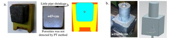
**Fig.1:** The views of the test EN-GJL 250 castings: a. standard DerTA cup (left), results of PT method after cutting (middle) and CAD geometry (right); b. real experimental cube casting (250 mm side) with upper riser \$\$\phi140x200\$ mm (casting and CAD geometry).
