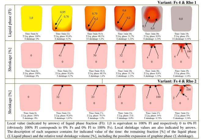
Table 2: Chosen results sequence obtained from NovaFlow&Solid CV for different variants: Fs & Rho.
