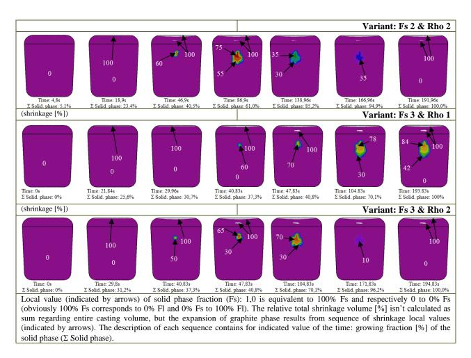
Table 4: Shrinkage sequence obtained from ProCast Micro model (to compare with Macro models).
