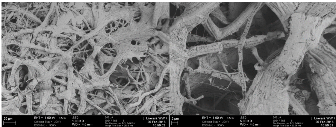
Figure 19. SEM micrograph of Zein/PCL after two weeks of degradation
