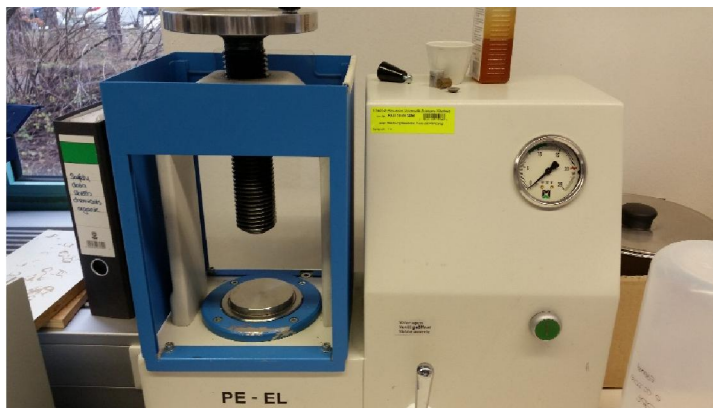
Figure 7. Image of the equipment used to make discs for FTIR analysis
