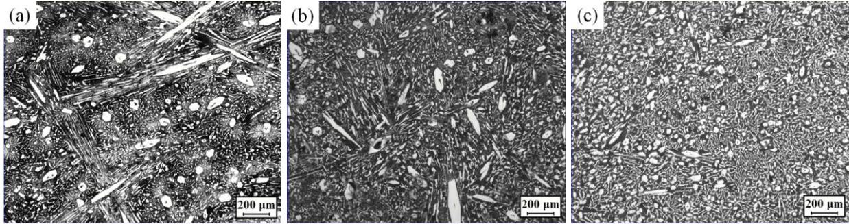
**Fig. 3:** Solidification microstructures from 1346 °C to  $T_e$  of the melts ECP treated for different time: (a) 0 min,  $T_e = 1346$  °C, (b) 1 min,  $T_e = 1337$  °C and (c) 2.5 min,  $T_e = 1327$  °C
