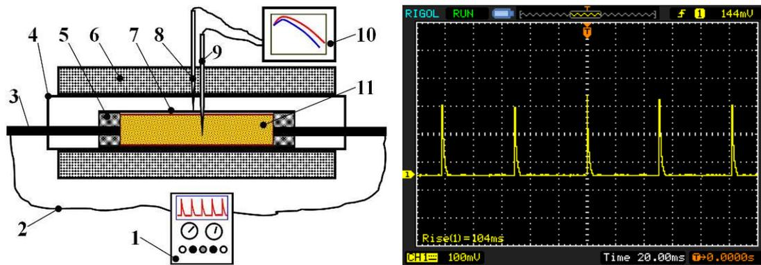
**Fig. 1:** schematic of ECP experiment: (a) experimental arrangement; (b) typical ECP waveform
