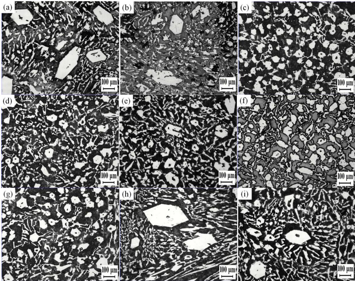
**Fig. 5:** Solidification microstructures from 1353 °C of the melts after treatment for 3.5 min at different ECP voltage, frequency, pulse width: (a) 500V, 15Hz, 10µs; (b) 500V, 30Hz, 30µs; (c) 500V, 45Hz, 100µs; (d) 1000V, 15Hz, 30µs; (e) 1000V, 30Hz, 100µs; (f) 1000V, 45Hz, 10µs; (g) 1400V, 15Hz, 100µs; (h) 1400V, 30Hz, 10µs and (i) 1400V, 45Hz, 30µs
