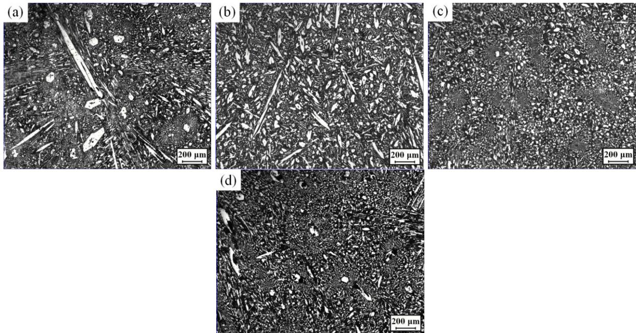
**Fig. 4:** Solidification microstructures from 1353 °C to  $T_e$  of the melts ECP treated for different time: (a) 0 min,  $T_e = 1353$  °C, (b) 2.5 min,  $T_e = 1351$  °C, (c) 3.5 min,  $T_e = 1346$  °C and (d) 5 min,  $T_e = 1336$  °C
