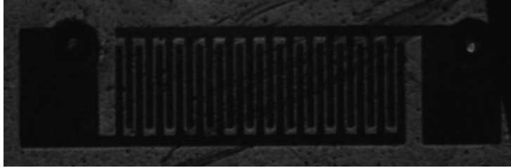
Figure 2.2: Pattern obtained after photolithography process (1.5x)
