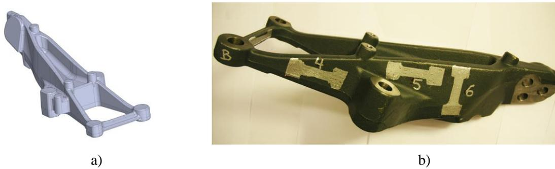
**Fig. 1:** a) CAD geometry of the engine support. 1b) Location of tensile test samples of the component. Tensile bar 1-4, 2-5 3-6 are located on each side of the component and 7 at the thin connection to the left.
